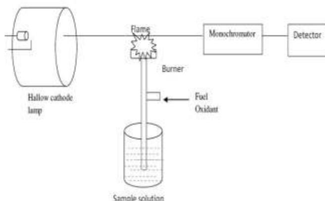
**Fig. 3: Atomic absorption spectroscopy** (<https://images.app.goo.gl/6FLRTq9rp62>)
