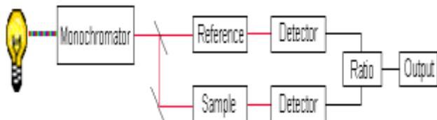
Fig. 5: Schematic Diagram of UV-Visible spectrophotometer
