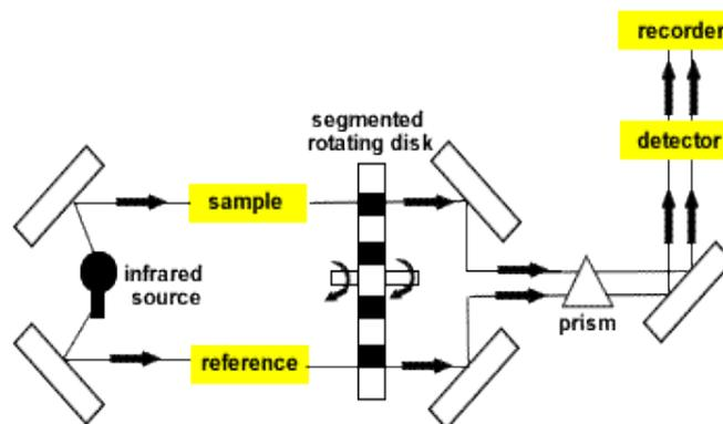
**Fig. 4: IR spectrophotometer**
